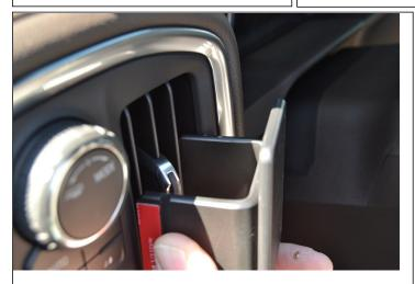
1. Clean the area where the ProClip will attach. The adhesive tape cover must be removed. Place the ProClip in your hand so the ProClip label (sticker) is in an upright position. Hook the notched right edge of the ProClip onto the right side frame around the far left dash vent.
