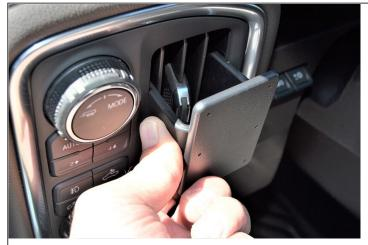
2. Press the left side of the ProClip to the right and hook the left notched edge of the ProClip onto the left side of the vent.
